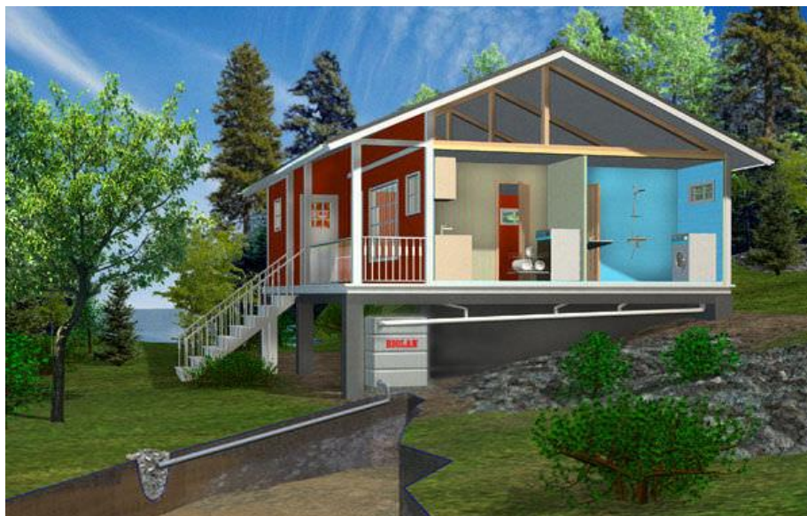
Figure 1.5: Waste/grey water system with an above ground tank
