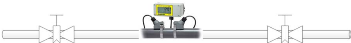
Figure 1.6: Ultrasonic (in-line) water flow equipment (non-invasive)
