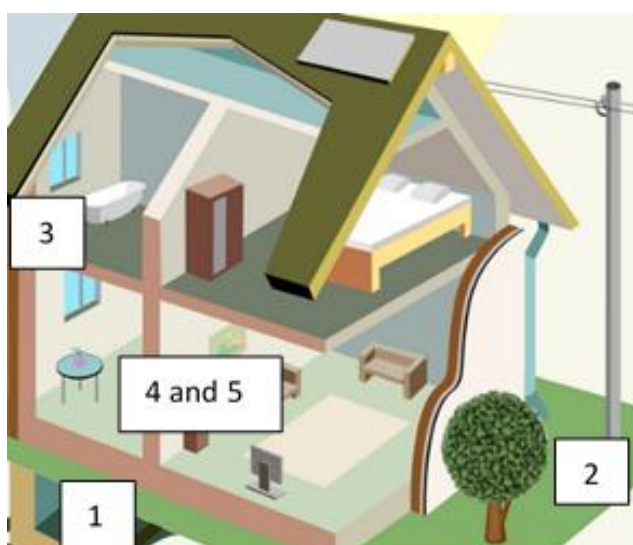
Figure 3.1: Five main areas in buildings: (1) water sources and infrastructure, (2) outdoor uses, (3) water fixtures, (4) water appliances, (5) domestic hot water production.
