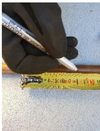
Figure 4.1: Correct tube measurement (left) & tube cutting (right). [Author: ST Spencer]
