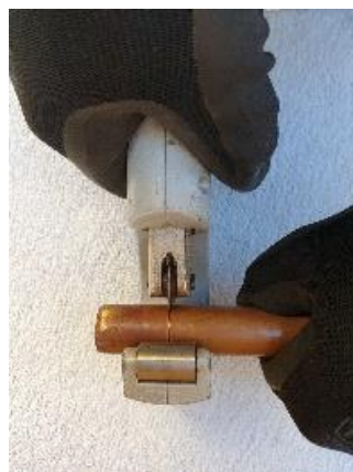
Figure 4.1: Correct tube measurement (left) & tube cutting (right). [Author: ST Spencer]
