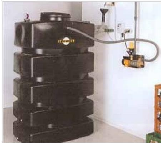
Figure 1.12: Indoor tank with capacity of 1500 litres, which can be increased by connecting several tanks in series, made of recyclable and non-deformable polyethylene
