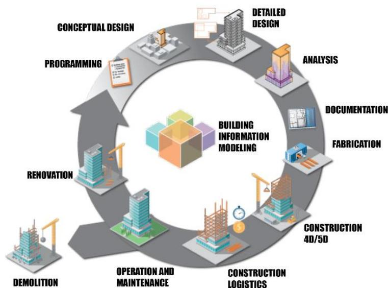
**Figure 2.2: BIM uses across building lifecycle**
