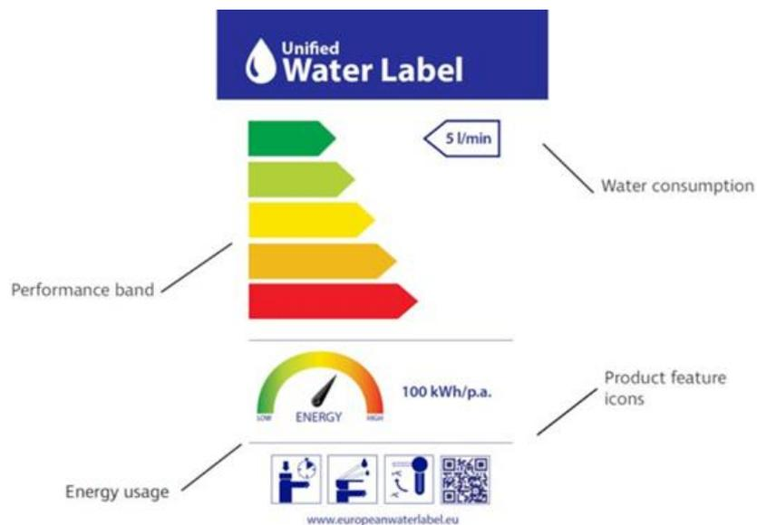
**Figure 2.4: Unified water label model**
