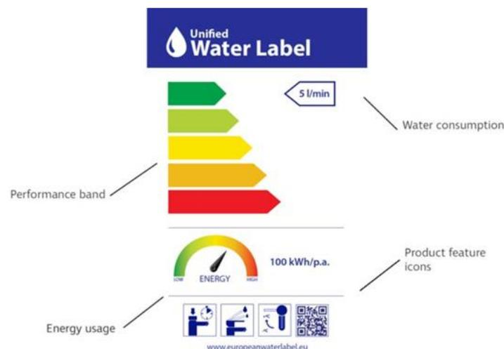
**Figure 1.6: Unified water label model**
