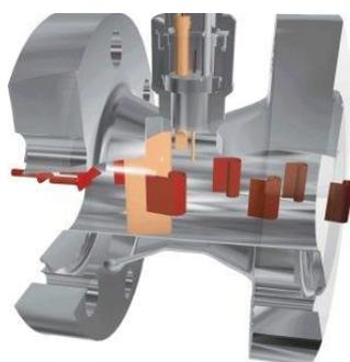
Ultrasonic flow meters measure the speed of fluid passing through the pipe using ultrasound to measure the volumetric flow. In a transit-time ultrasonic liquid flow meter, an ultrasonic signal is
