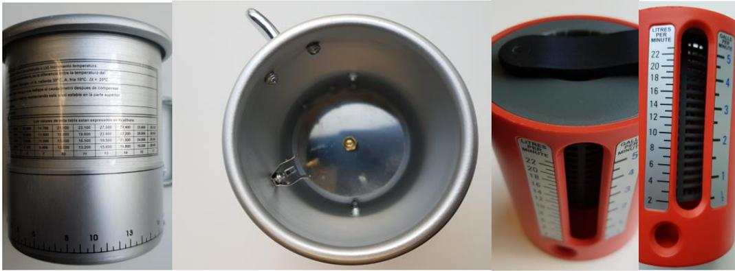
**Figure 1.9: Flowmeter equipment to measure the flow at fixtures**
