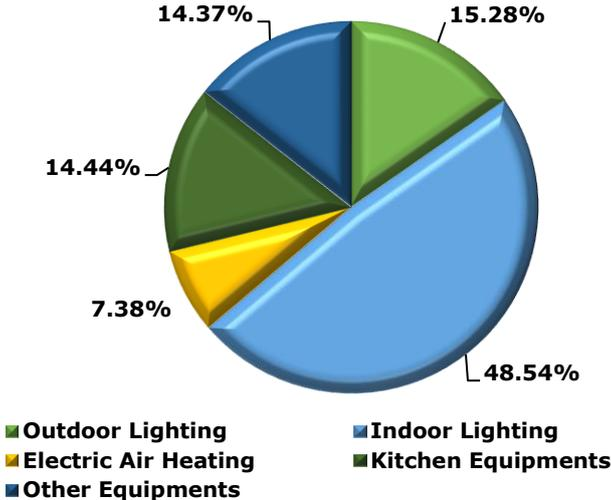
**Figure 3.5: Example of a system breakdown of energy consumption that may ideally occur in an educational building**
