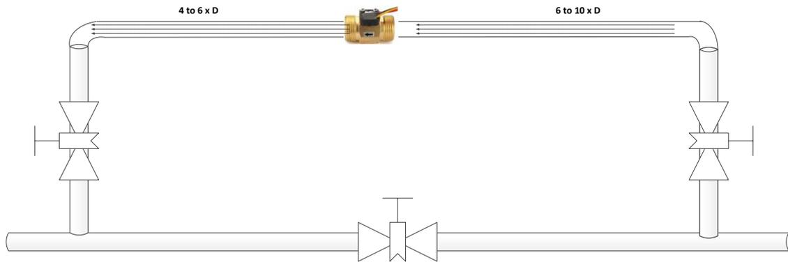
**Figure 1.12: Mechanical water flow equipment (invasive)**
