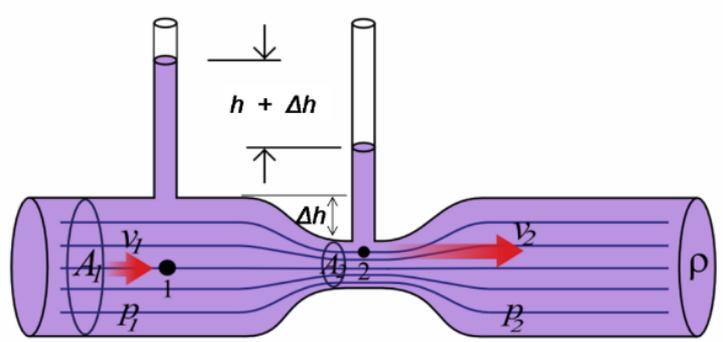
**Figure 1.2: Working principle of venturi flowmeter**
