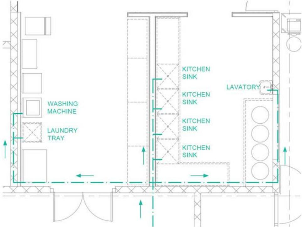
**Figure 1.6: Example of a domestic water distribution system for a commercial kitchen**
