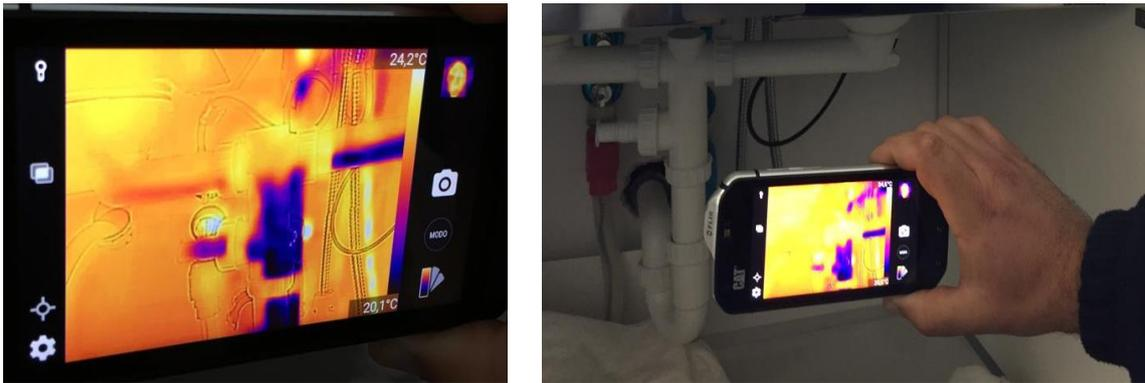
**Figure 1.10: Thermographic equipment to measure temperature differences**
